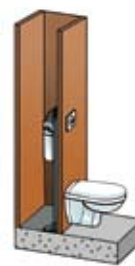
Installation en gaine technique
